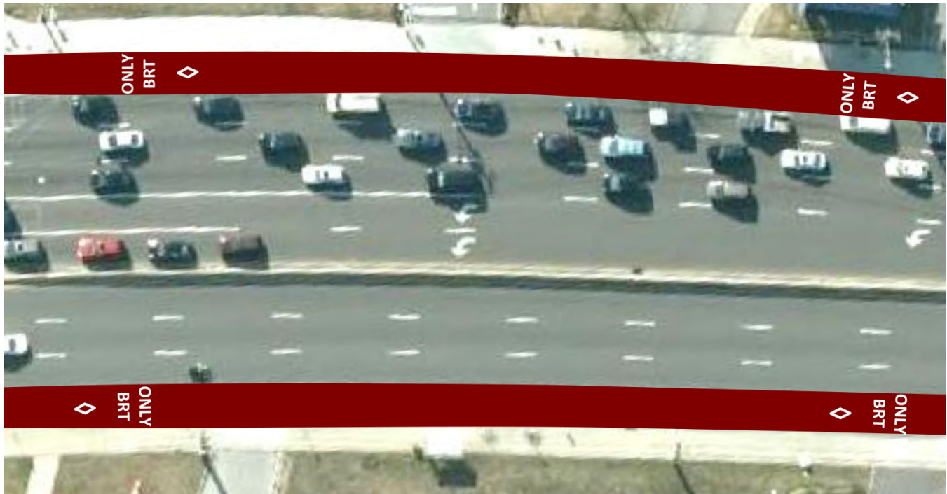
FIGURE 34: Sample BRT Lane Colored Pavement Treatment
